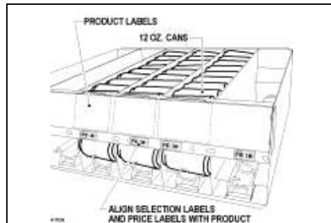
Figure 5d. Loading Dispenser Mechanism
